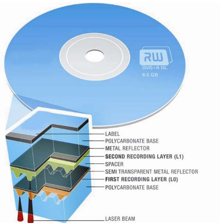
Figure 1 – Cross Section of a DVD+R DL Double Layer Disc
